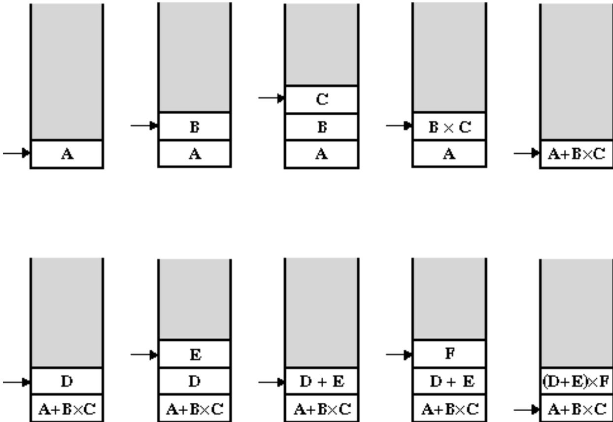
The final step combines the top two stack elements using the + operator.
