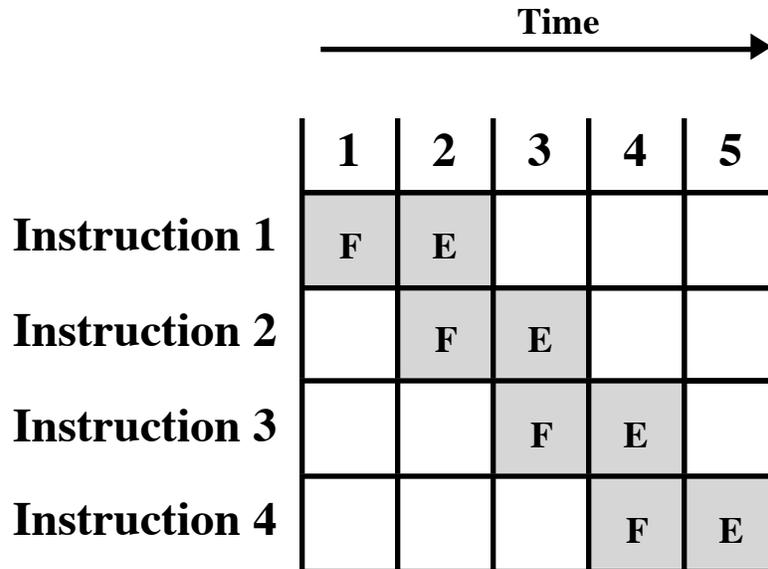
This diagram distorts the true picture. The execute stage will be much longer than the fetch stage.
